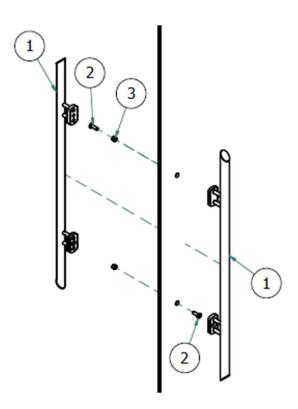
Figure 17: STEP 7 - Glass handle assembly
