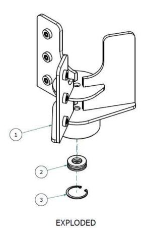
Figure 13: STEP 4 - Base spider assembly
