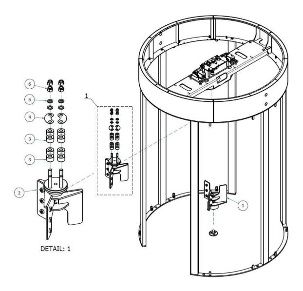
Figure 14: STEP 5 - Glass spider clamps assembly
