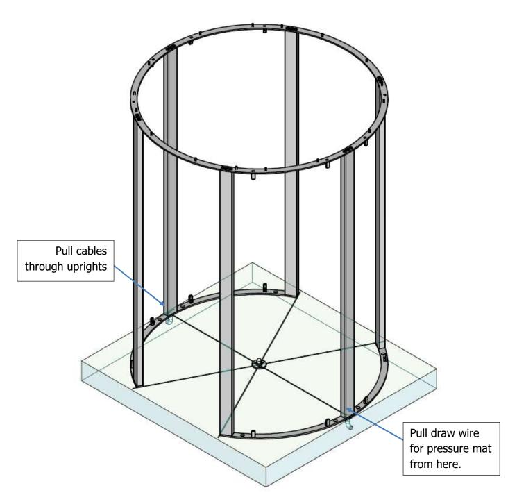
Figure 10: Frame assembly on plinth
