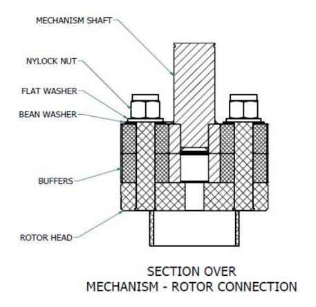
Figure 15: Top spider assembly to mechanism shaft
