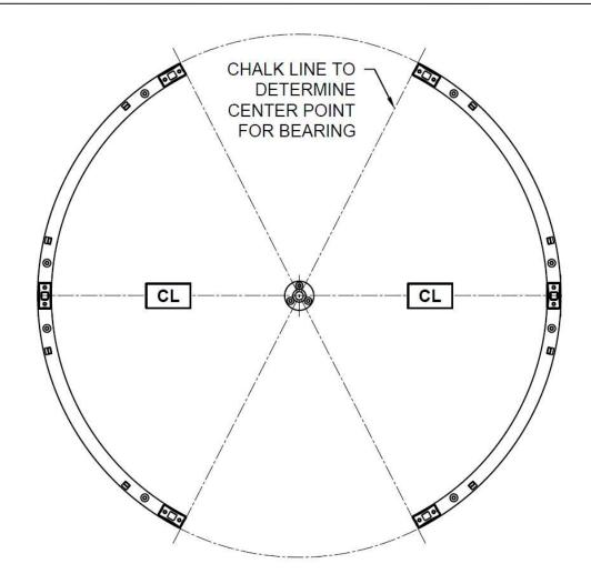
Figure 12: Marking for bearing plate
