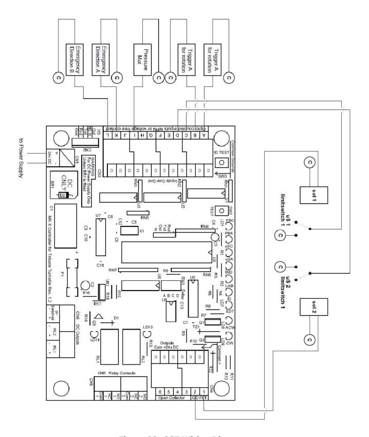
Figure 23: CGT Wiring Diagram
