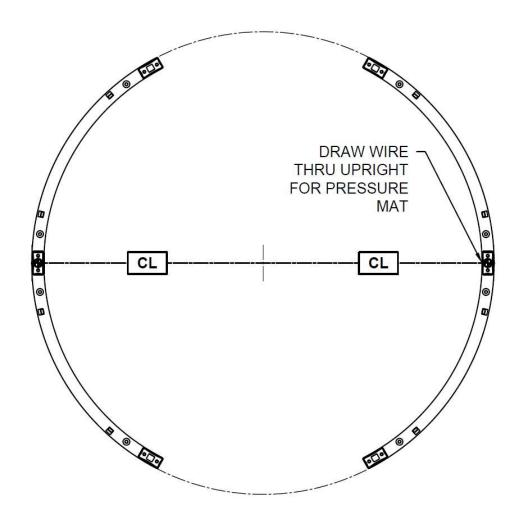
**Figure 8: Frame placement**
