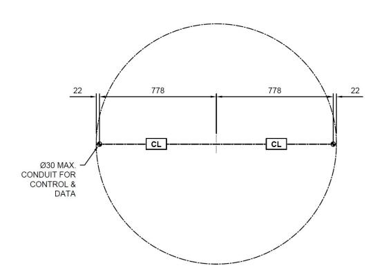
Figure 6: Marking the floor: Step 3
