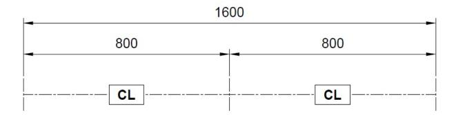
Figure 4: Marking the floor: Step 1
