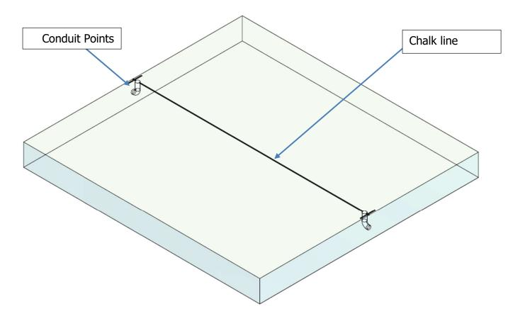
Figure 3: Isometric view of plinth
