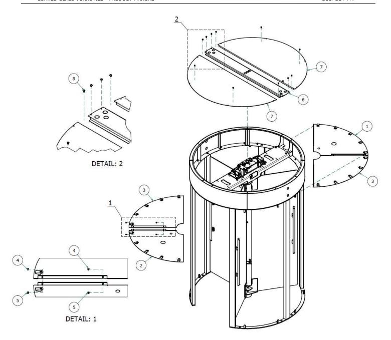
Figure 19: STEP 8 - Ceiling and roof assembly
