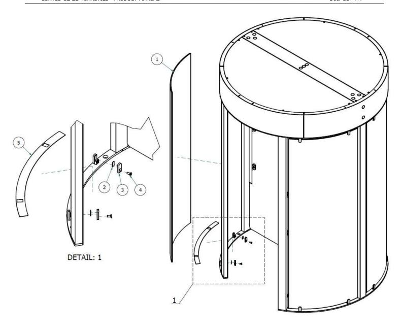
Figure 21: STEP 9 - Side Glass Assembly
