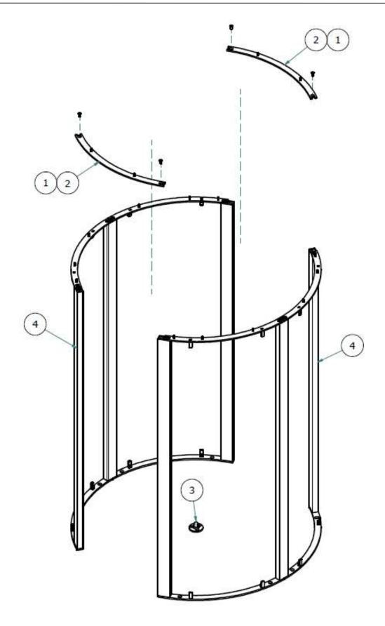
Figure 9: STEP 2 - Frame assembly
