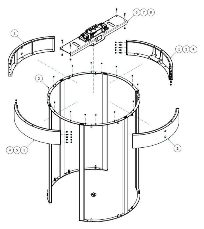
Figure 11: STEP 3 - Crown & Drive channel assembly
